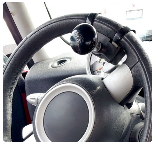
Installing a spinner knob on your car's steering wheel may be required if stipulated during an assessment.
